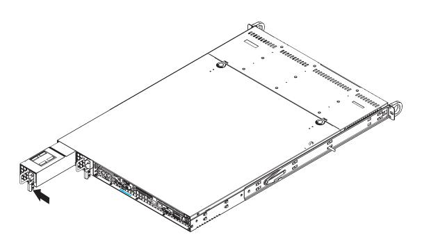
Figure 6-6. Removing/Replacing the Power Supply
